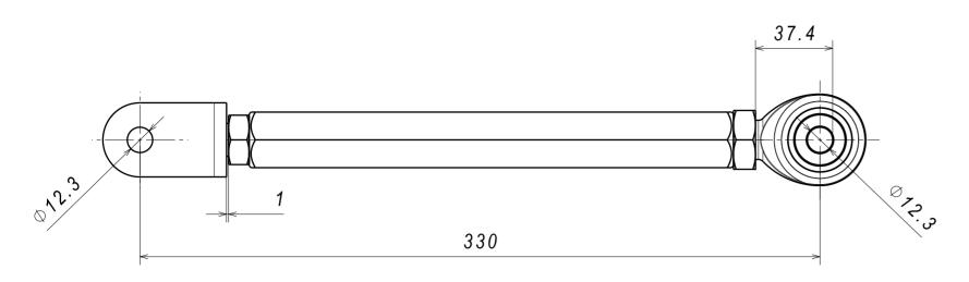
MINIMUM LENGTH - 330 mm (MEASURED BETWEEN HOLE CENTERS)
