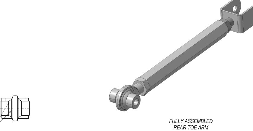
CHECK FOR ROD END BEARING ALIGNMENT AFTER TIGHTENING THE ADJUSTING MECHANISM IT MUST BE PARALLEL TO THE BODY OF THE ROD END
