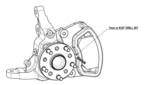
6. INSTALL CHOSEN FRONT ROTOR SOLUTION AND CONFIRM CLEARANCE BETWEEN ROTOR HAT AND CALIPER
