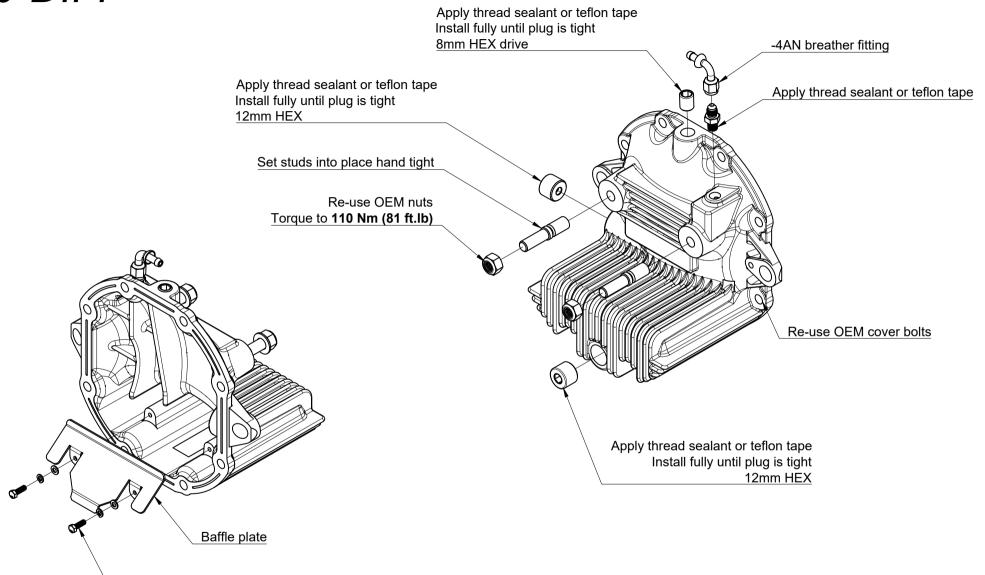
Install using **high strength** thread locker (Loctite 263) or equivalent Torque to **10Nm (7.4 ft.lb)**
