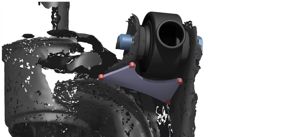
Image 8. Camber arm brace spot welds
