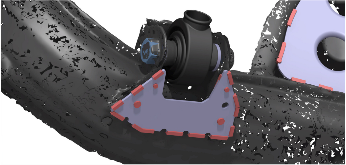
Image 13. Lower control arm rear bracket brace stitch welds
