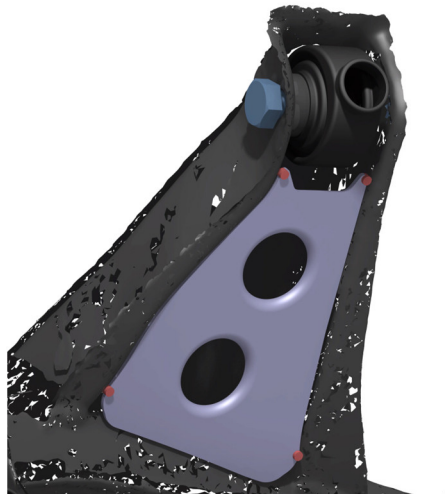
Image 10. Traction arm brace spot welds
