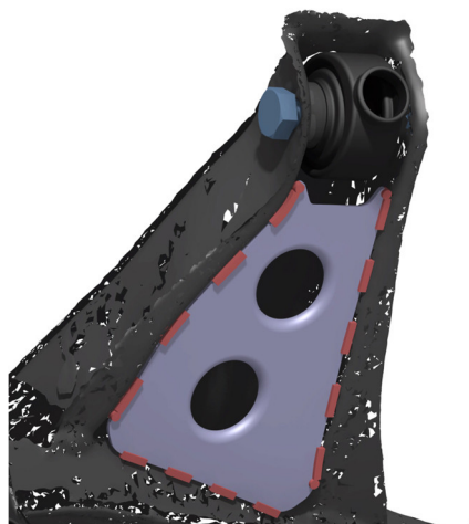
Image 11. Traction arm brace stitch welds
