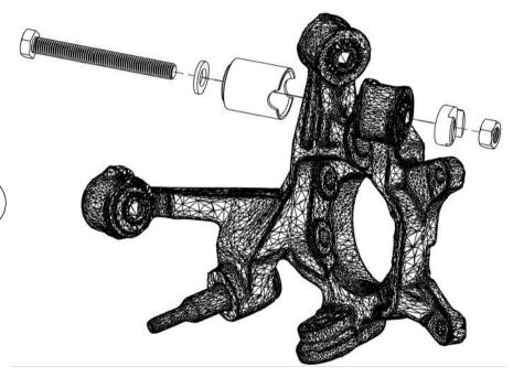
3. TIGHTEN THE HEAD OF THE BOLT UNTIL THE BUSH IS FULLY PULLED INTO THE CLEARANCE CUP. THE ASSEMBLY WILL THEN COME LOOSE.
