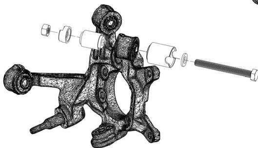
3. SLOWLY TIGHTEN THE BOLT HEAD, MAKING ADJUSTMENTS TO KEEP THE BUSH ALIGNED WHERE NECESSARY.
